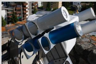
The Precision Filter Radiometer (PFR) is a research grade instrument to measure direct solar irradiance in 4 narrow spectral bands centered at wavelengths recommended by World Meteorological Organization for the determination of atmospheric aerosol optical depth (AOD).
