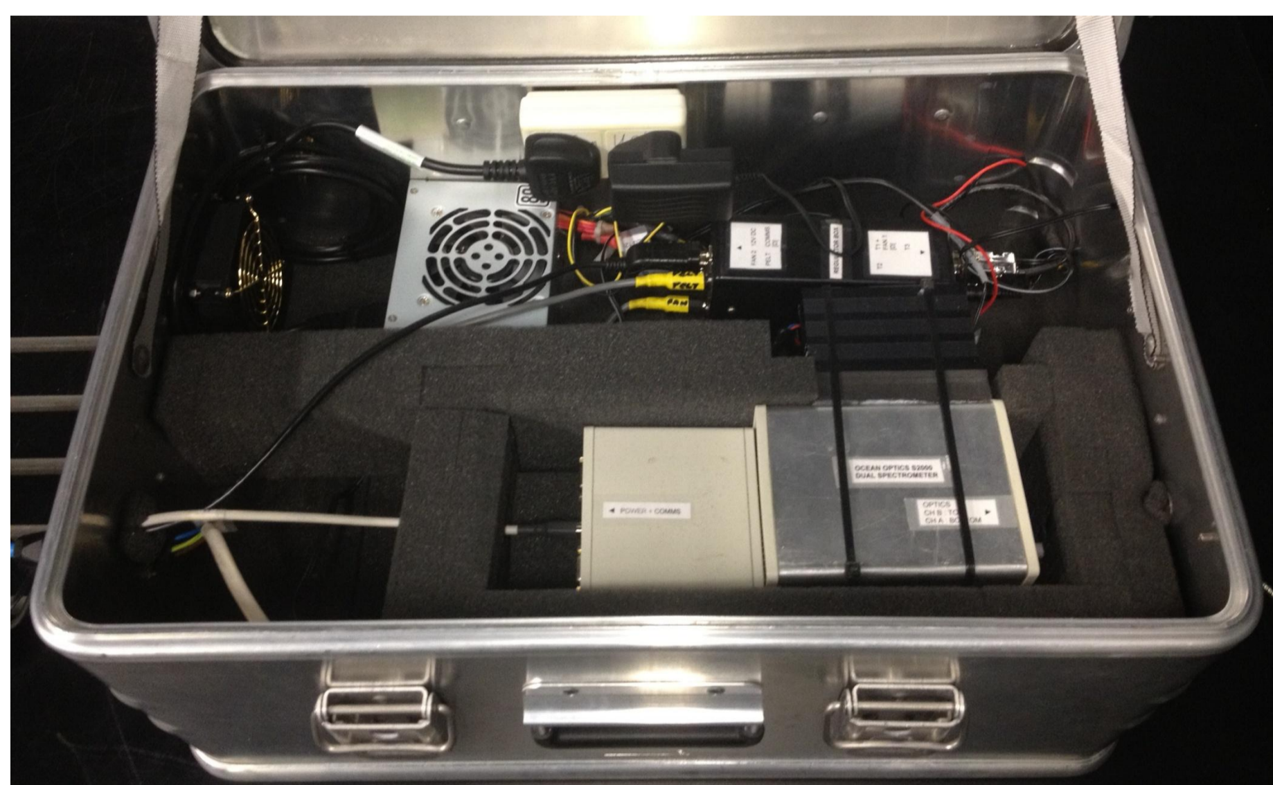
Weatherproof housing for Ocean Optics S2000 dual channel spectrometer
