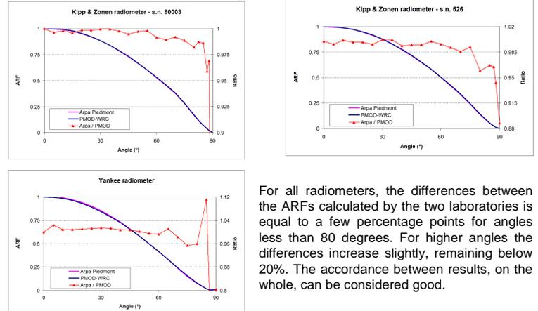
For all radiometers, the differences between the ARFs calculated by the two laboratories is equal to a few percentage points for angles less than 80 degrees. For higher angles the differences increase slightly, remaining below 20%. The accordance between results, on the whole, can be considered good.
