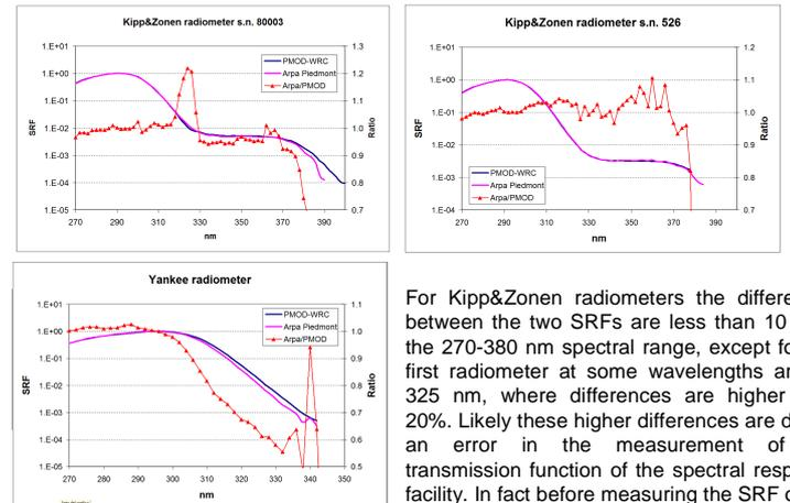
For Kipp&Zonen radiometers the differences between the two SRFs are less than 10 % in the 270-380 nm spectral range, except for the first radiometer at some wavelengths around 325 nm, where differences are higher than 20%. Likely these higher differences are due to an error in the measurement of the transmission function of the spectral response facility. In fact before measuring the SRF of the
