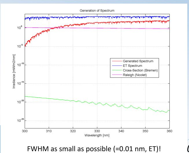
**1. Generating spectrum** (PMOD-model) between **300 – 360 nm** with known parameters and 49 atmosperic conditions 7 ozone x 7 airmass  $I_{\lambda} = I_{\lambda}^{0} e^{-\tau_{\lambda} m}$
