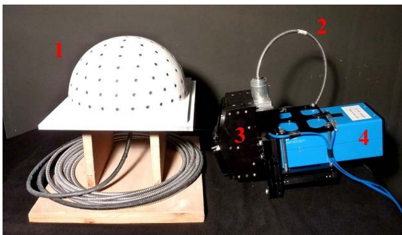
Figure 1. Main components of MUDIS: hemispherical entrance optics dome with weather protection (1), fibre bundle (2), Offner imaging spectrometer (3), UV-sensitive CCD camera (4).
