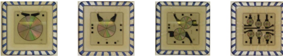
Figure 1: Photographs of the AlN MSM photodiodes mounted on ceramic packaging. The MSM area are (from left to right) 4, 3, 2 and 1 mm diameter with 2 \mu m interdigitated finger width and 5 \mu m spacing between two electrodes.
