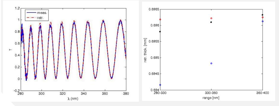
From a set of calibrated instruments (in a limited spectral region) the actual thickness is retrieved off-line
