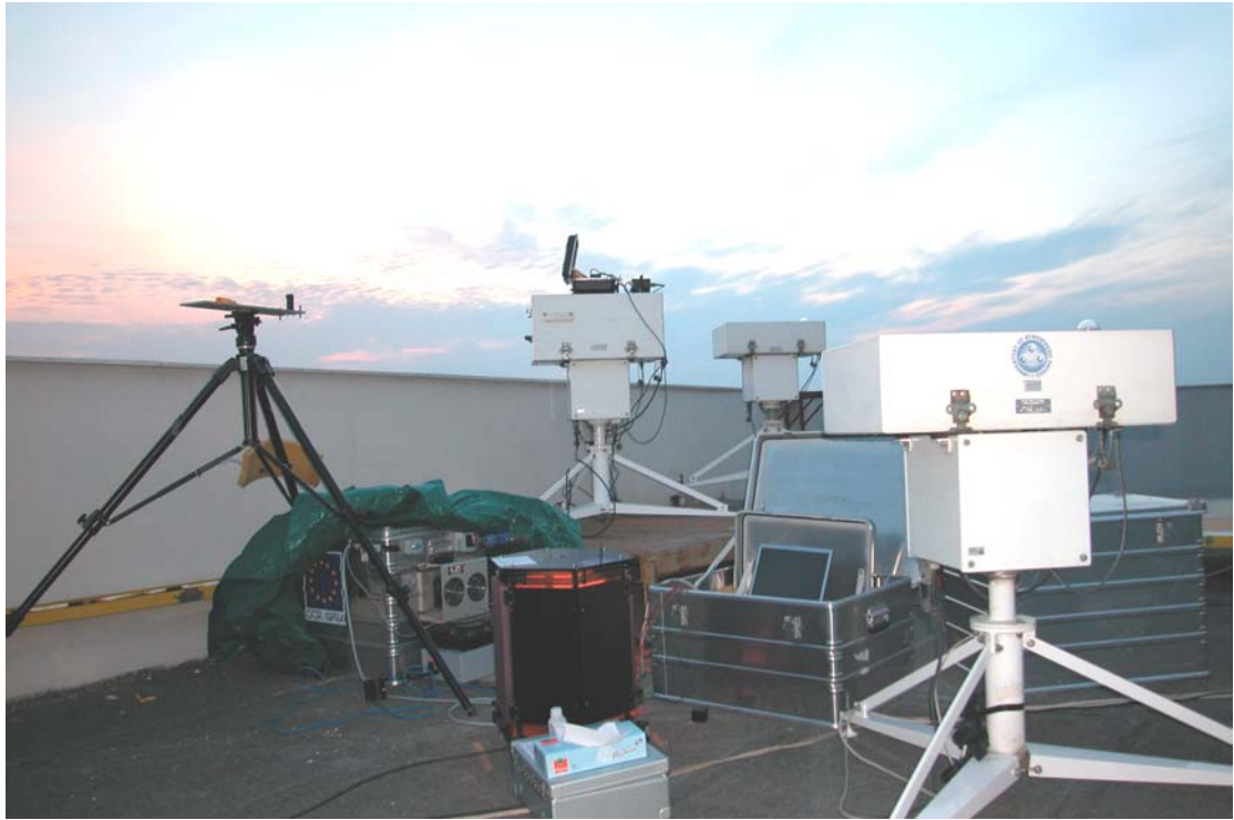
Figure 3 Measurement setup, LAP, Thessaloniki, October 5, 2002 at 7 PM. B5503 left, Brewer #086 at center background.
