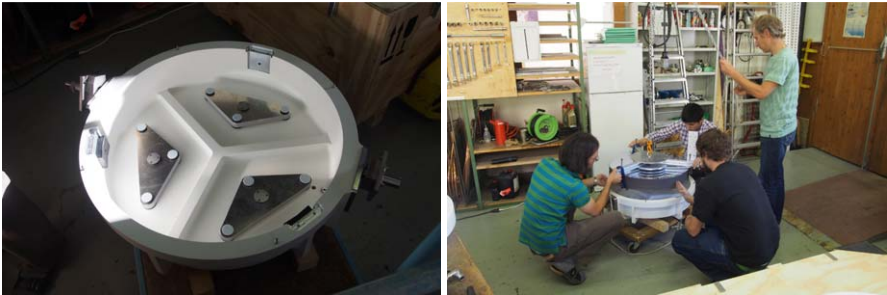
Figure 7.2: Empty mirror support frame (left) and integration of the mirror into the support frame (right).
